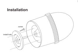
Fix the bottom support to the wall first, then install the unit to support.
