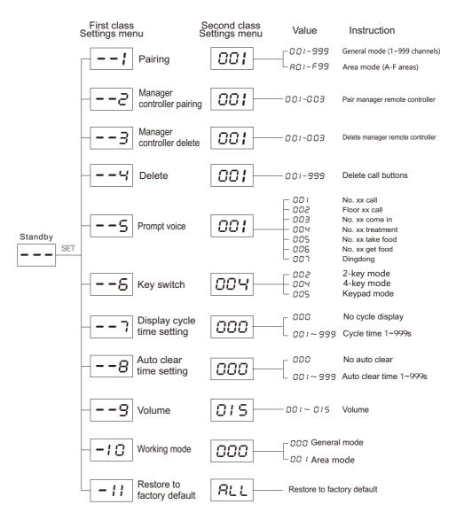
Note: According to the transmitter type, select the key mode (--6) first, then select the suitable working mode (-10) and prompt voice (--5), at last pair the transmitters.
